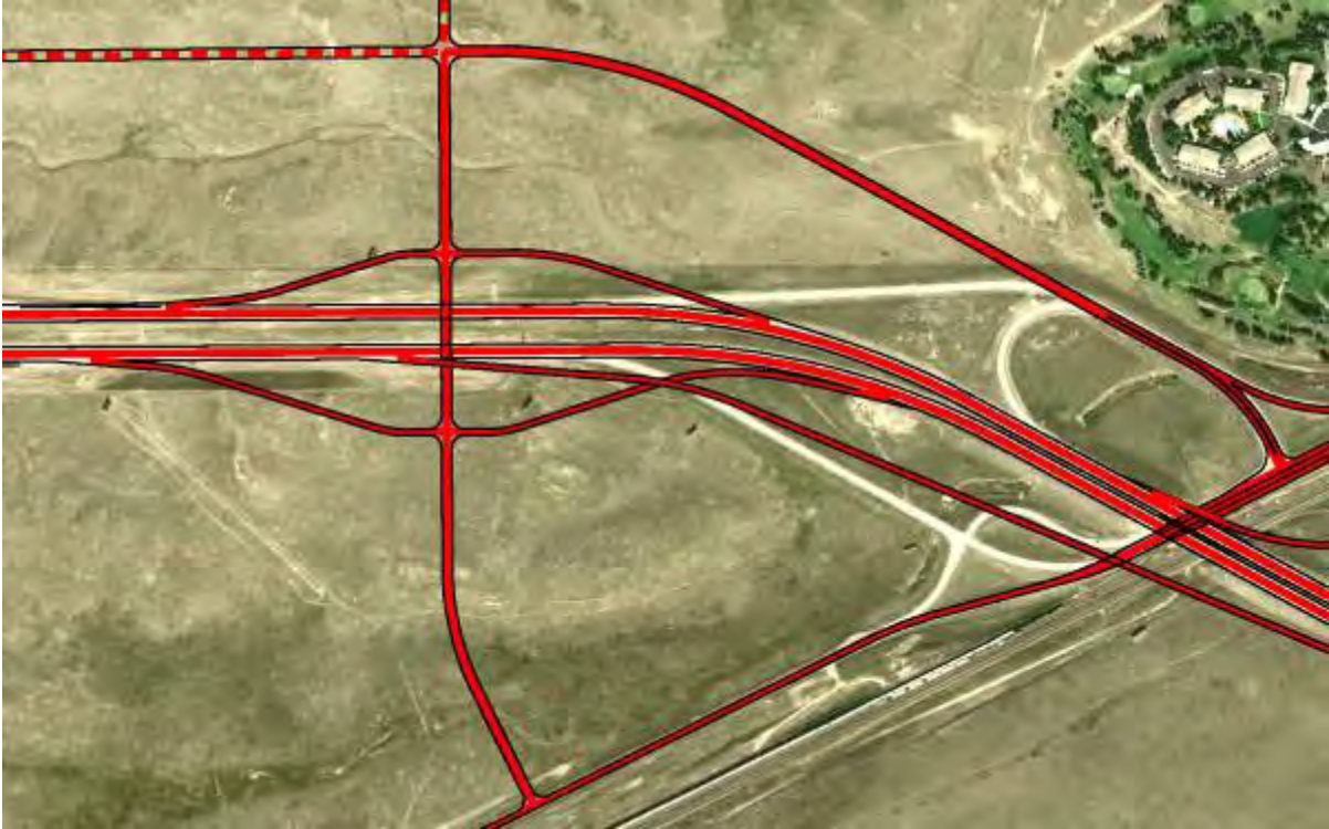
Figure 22 - Alternative B5 – Diamond
