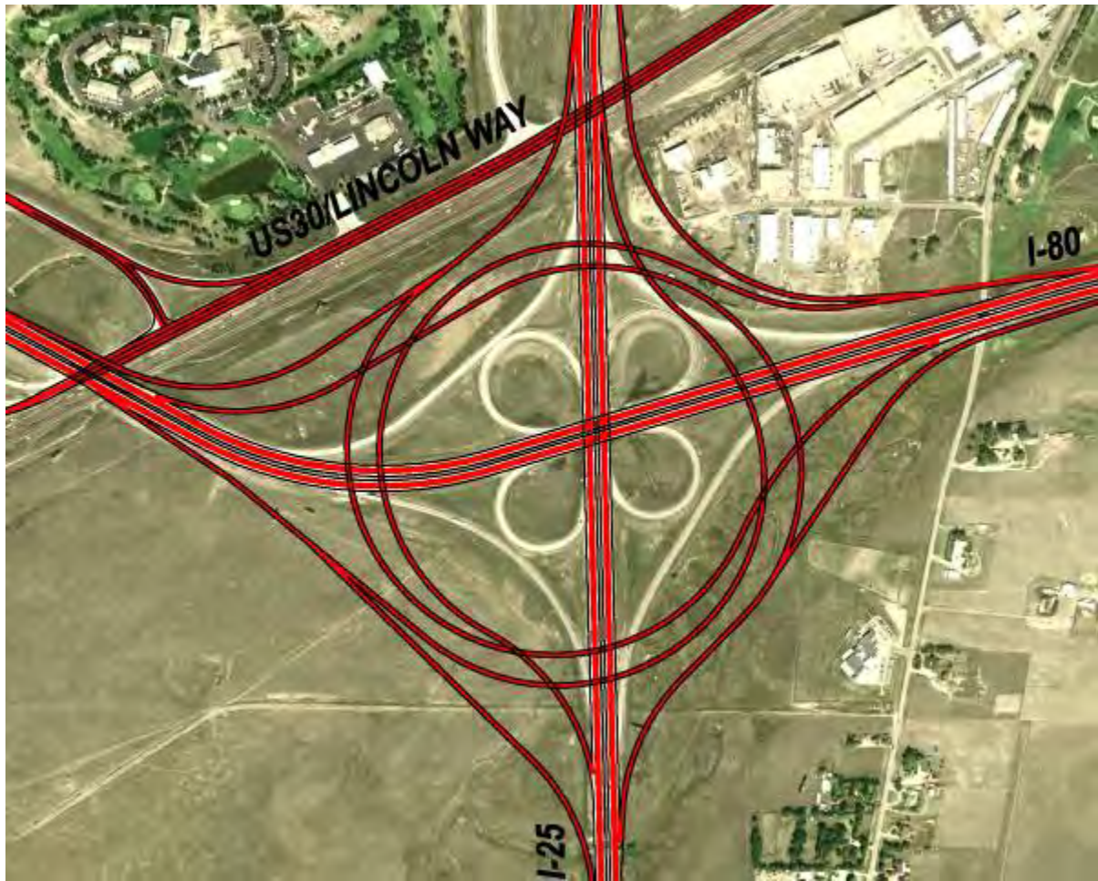
Figure 11 - Alternative IV – Full Turban
