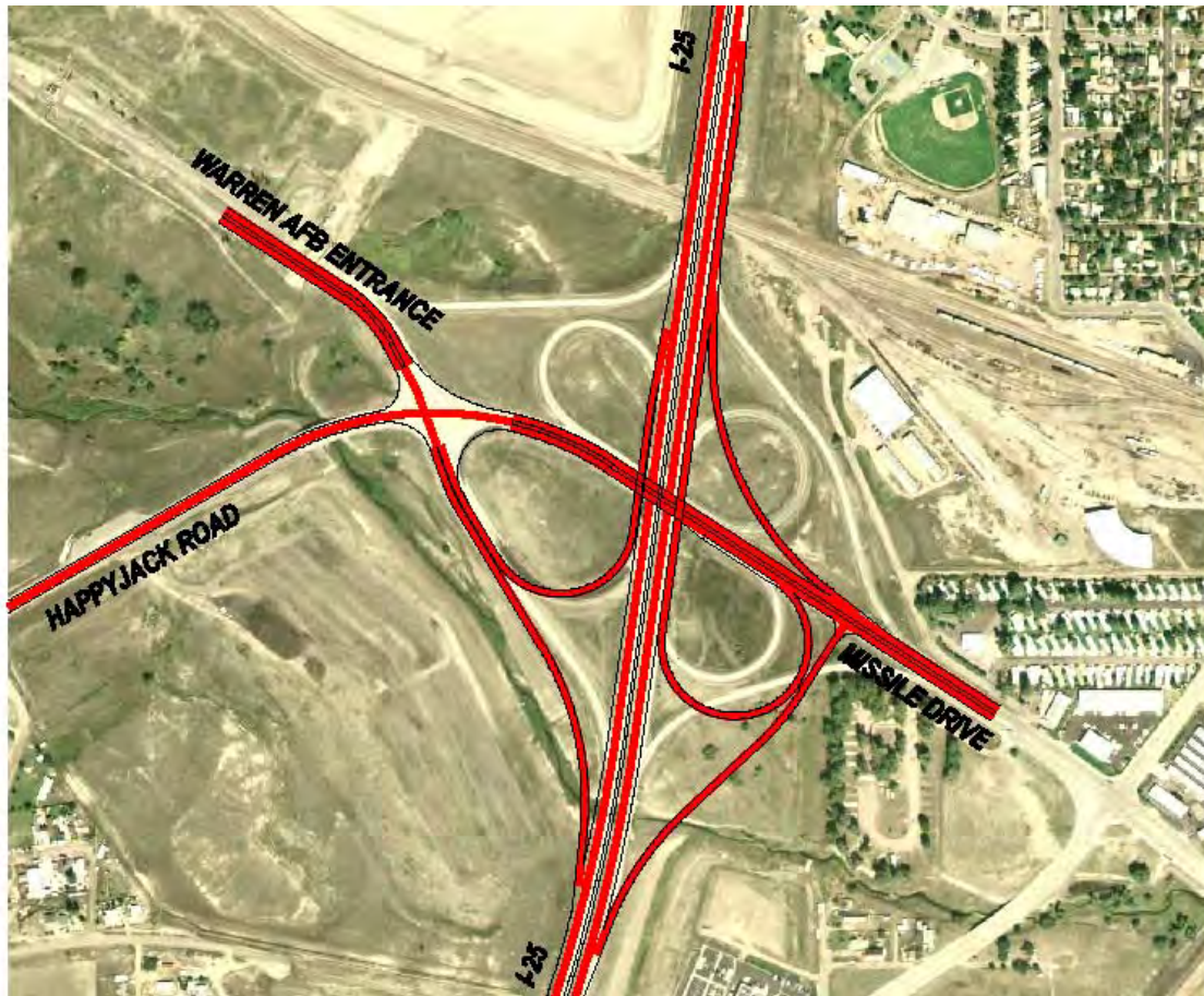
Figure 26 - Alternative D2 – PARCLO A/B
