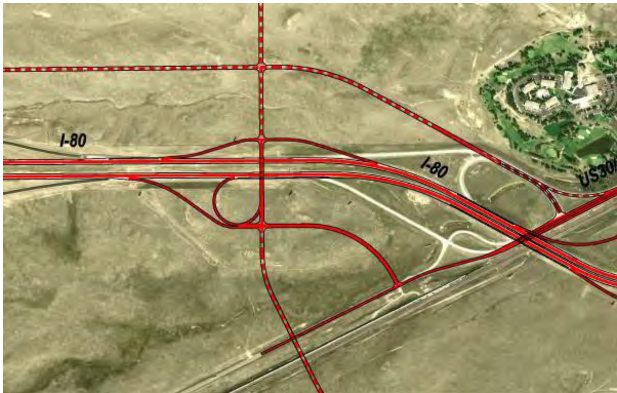
Figure 18 - Alternative B1 – Diamond with Single Loop
