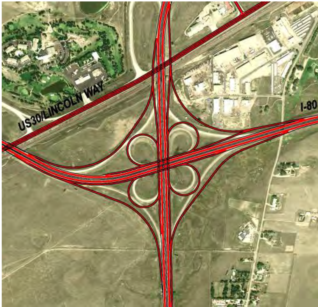
Figure 12 - Alternative V – Full Cloverleaf with Connector-Distributor (CD) Roads
