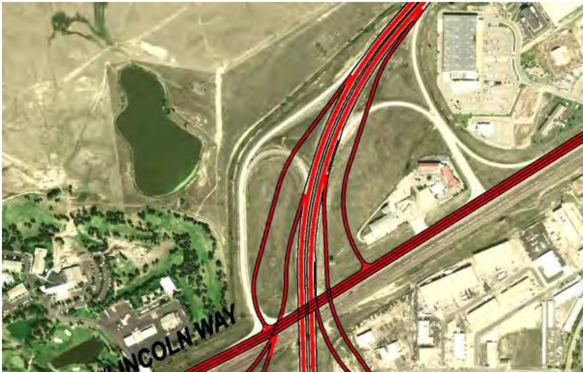
Figure 14 - Alternative A1 – Half Diamond Existing Location
