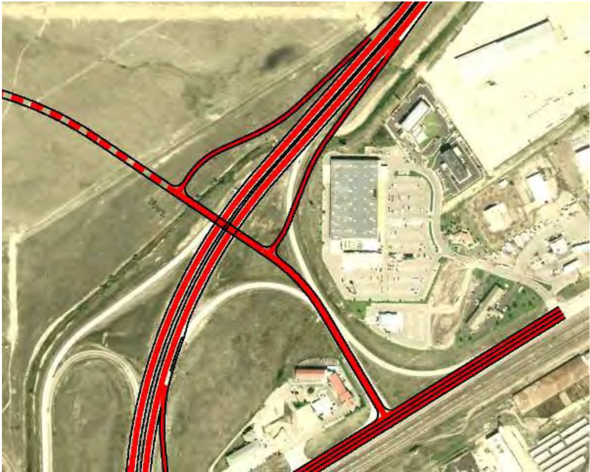
Figure 17 - Alternative A4 – Half Diamond Relocated
