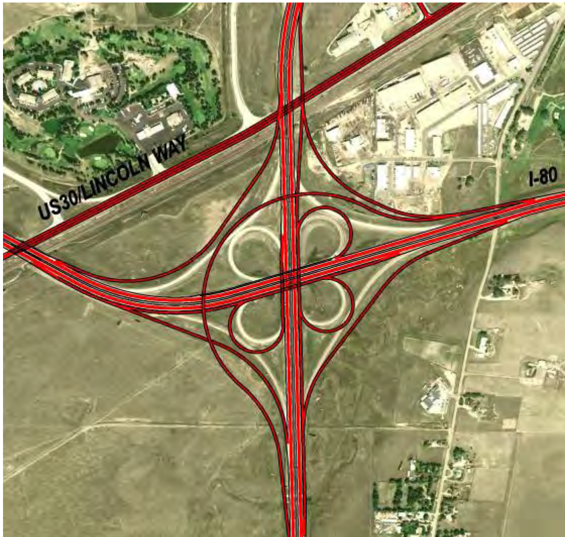
Figure 13 - Alternative VI – \frac{3}{4} Cloverleaf with CD Roads and Flyover
