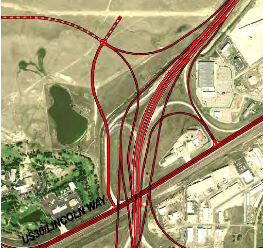
Figure 16 - Alternative A3 – Hook Ramps
