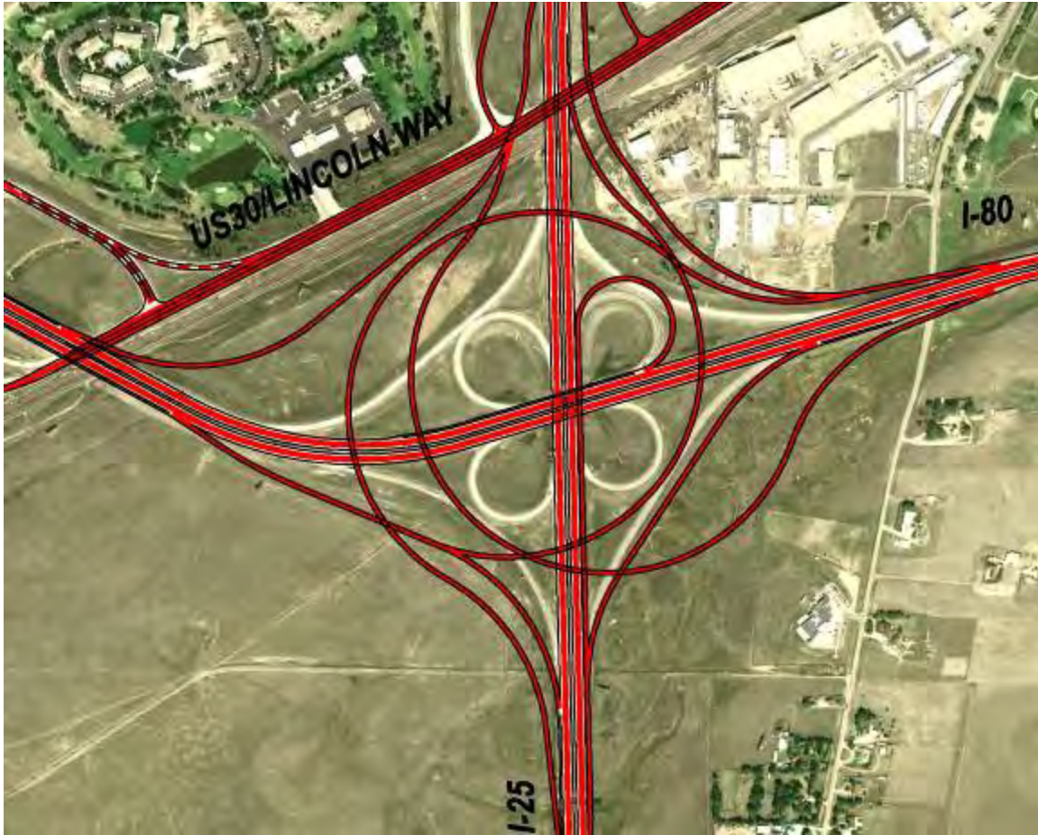
Figure 8 - Alternative I – Single Loop with Turban
