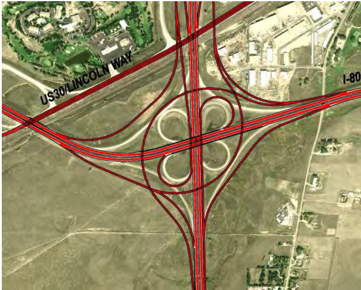
Figure 9 - Alternative II – Double Loop
