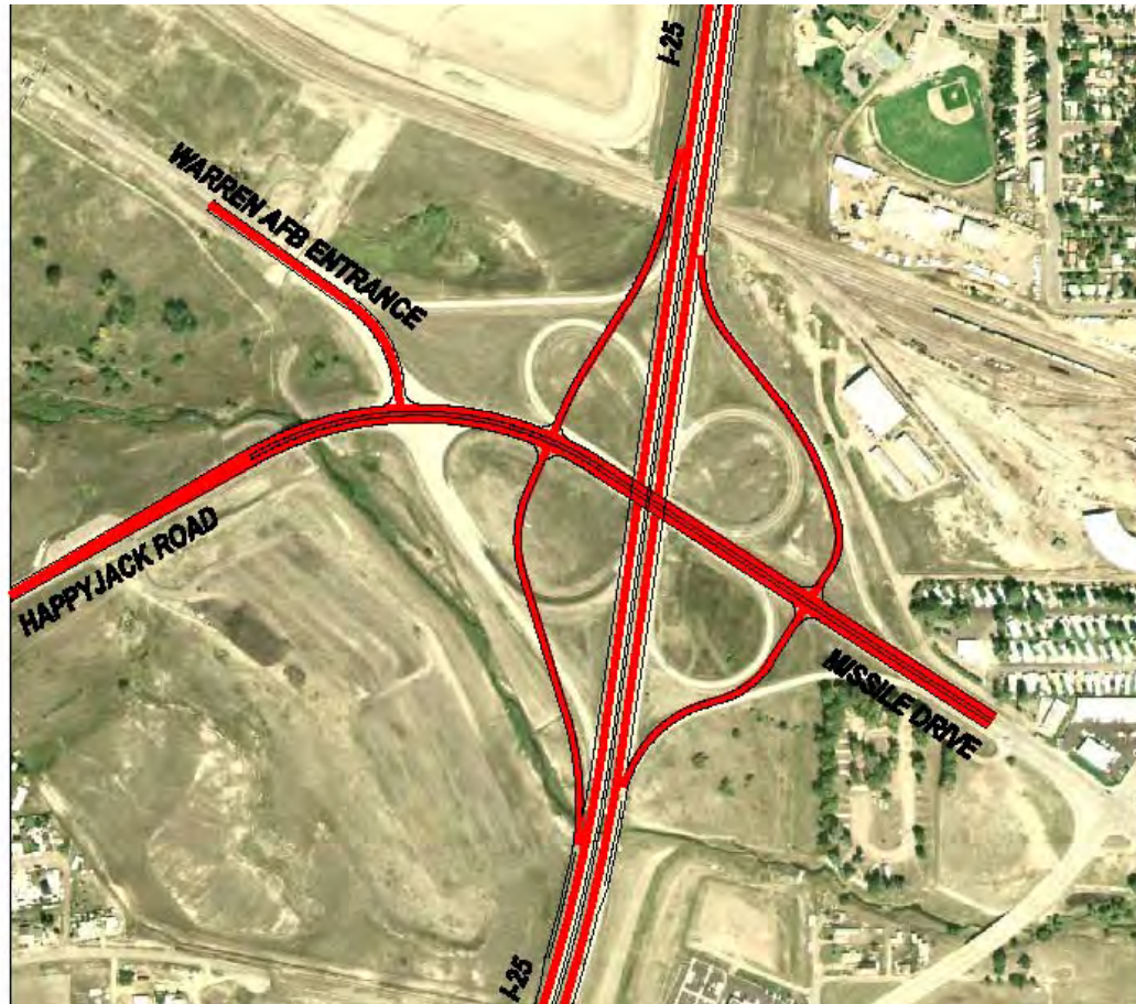
Figure 25 - Alternative D1 – Diamond
