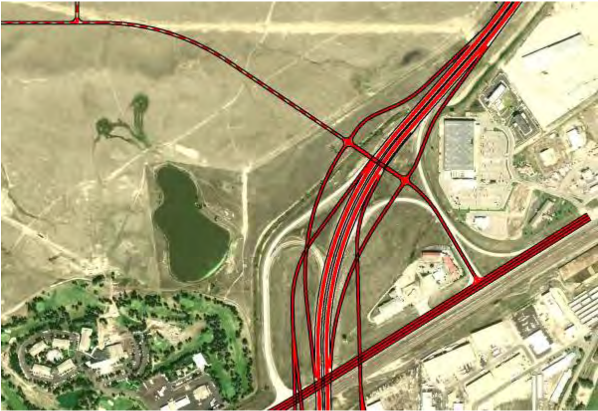
Figure 15 - Alternative A2 – Full Diamond with Braided Ramps
