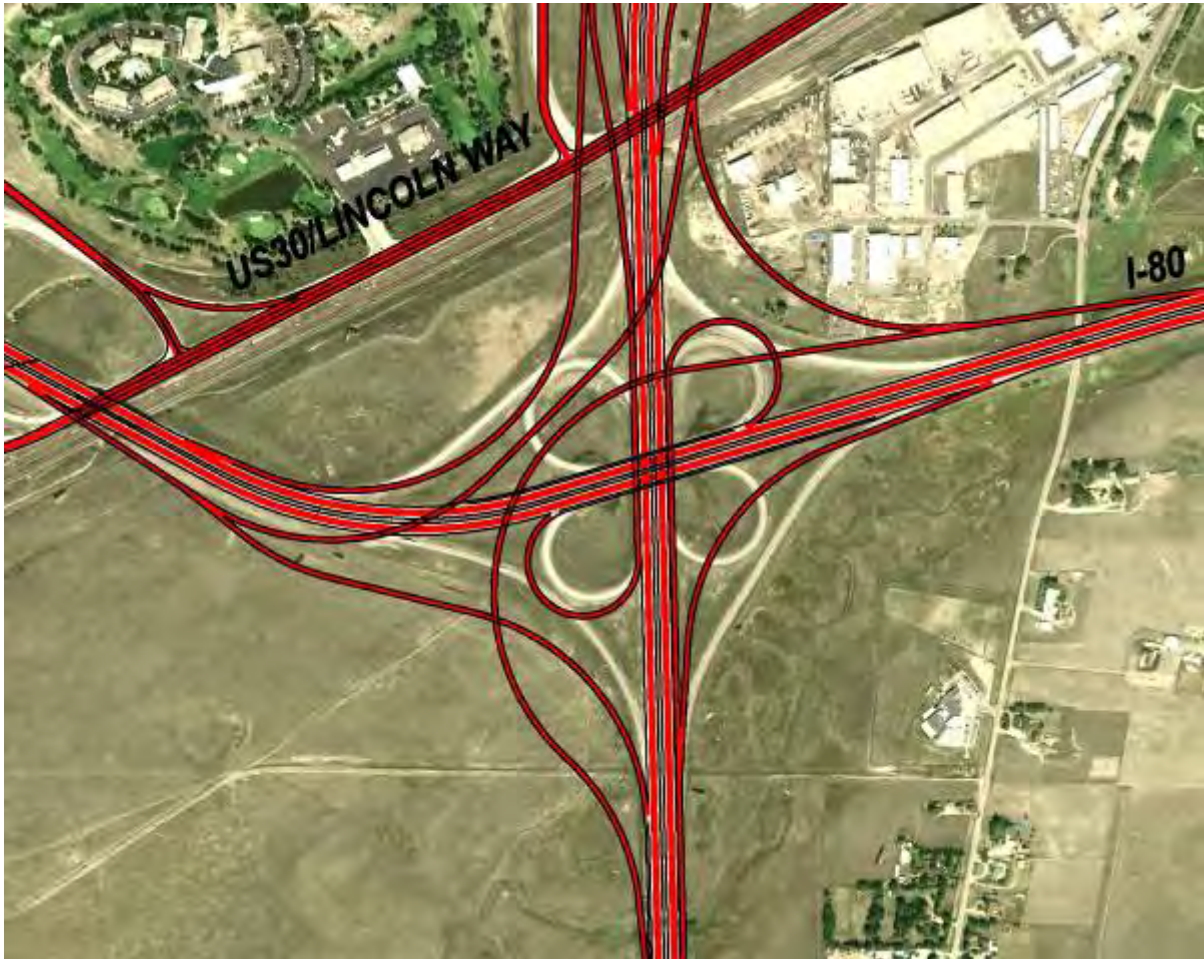
Figure 10 - Alternative III – Stack
