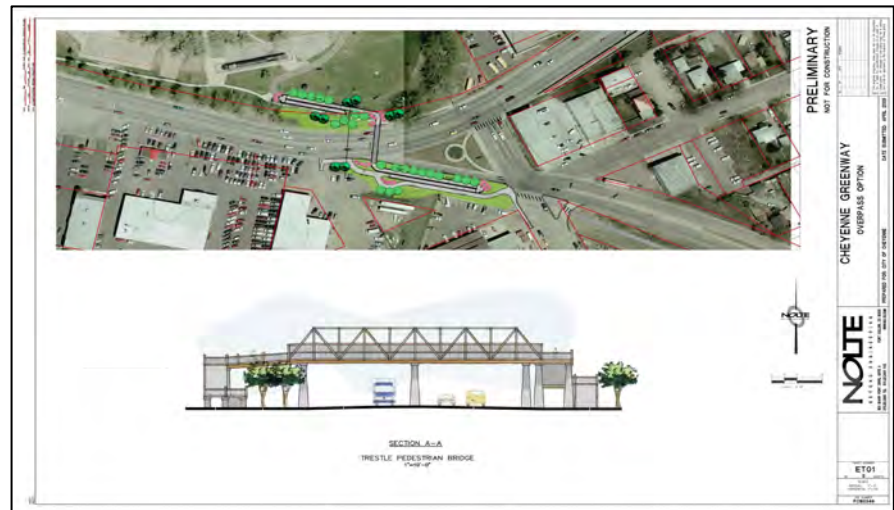
Figure IV.A.4, Option 3 Overpass Concept
