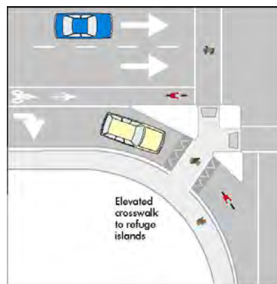
Figure 8-9. Elevated Crosswalk to Refuge Islands
