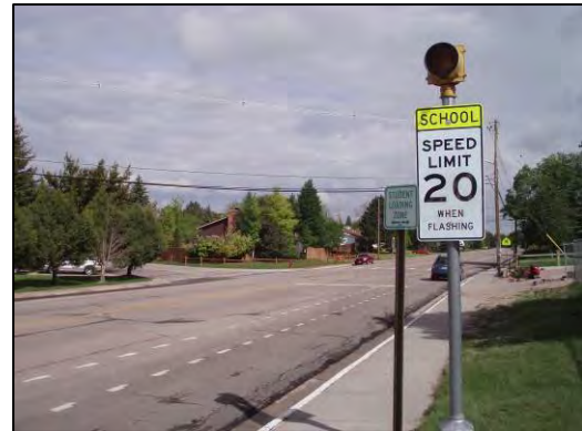
Figure 15. Flashing warning lights and signage can remind drivers to watch for pedestrians and bicyclists in School Zones
