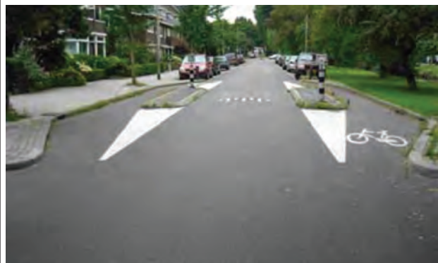
Figure 37. Example of a pinch point treatment.
