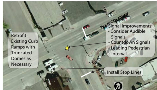
Proposed intersection improvements at Ames Avenue and West Lincolnway. Suggested improvements include moving the signal controller box in the middle of the sidewalk on the SE corner of the intersection.
