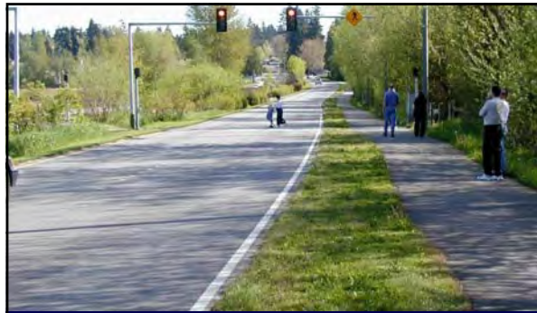
2-step signal for trail crossing Phase 1: users cross stopped traffic
