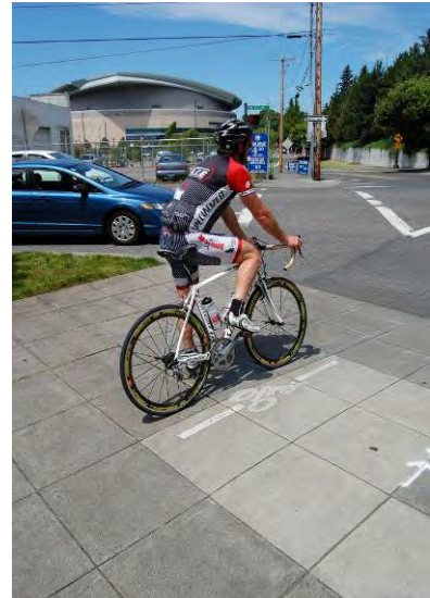
Figure 15. Traffic signals can be activated by in-pavement signal loops. Pavement markings guide cyclists in correct placement of their bicycle to trigger the traffic signal.
