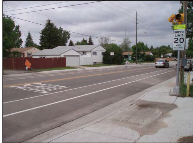
Figure 22. Bike lanes, School Zone warning signs and pavement markings increase the safety of students using 12th Street to access Bain Elementary
