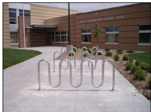
Figure 61. Bike parking located near a building entrance can provide secure and safe bicycle parking for students.
