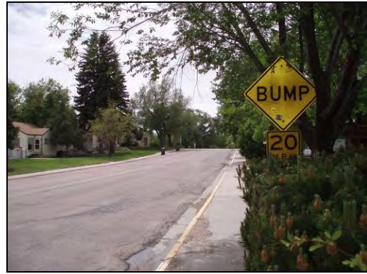
Figure 7. Overgrown vegetation impedes pedestrian travel on sidewalks
