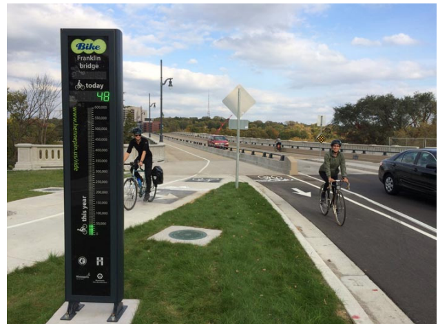
Figure 33: Manual and automated count programs (Credit: Minnesota Department of Transportation, University of Minnesota Center for Transportation Studies)
